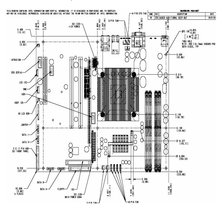
Figure 11. SE7221BK1-E Server Board Mechanical Drawing
